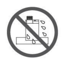
Electrical parts such as motor, switch and connector must not be damped by water. Do not clean the range hood with water. Do not use the range hood after it becomes wet as accidents such as electric leakage and electric shock may occur.
