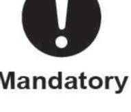
Do not connect this product to a long patch board. If the cable is long, fire Mandatory hazard or electric leakage may be caused by overheated cable when the oven is working.
